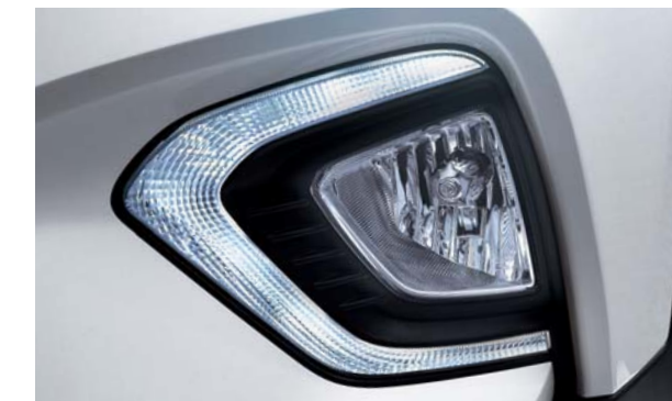
Fog lamp with LED daytime running lights (DRL)
